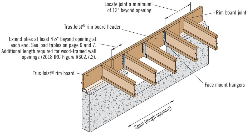
*Support TJ® joists from rim board header with face mount hangers only. For 1-ply header applications, reduce hanger capacities according to hanger manufacturer's recommendations.*
